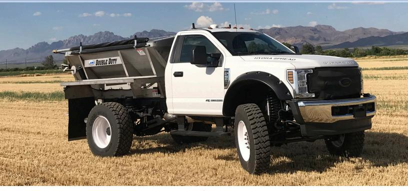
The GVM Hydra Spread was designed to offer versatility and maneuverability to custom applicators, co-ops, and farmers. GVM's Hydra Spread pairs a Ford F-550 chassis with our reliable and accurate Double Duty spreader body, provides a narrow, mechanical drive machine with a tight turning radius, comfortable road travel, and an unbeatable spread pattern.
